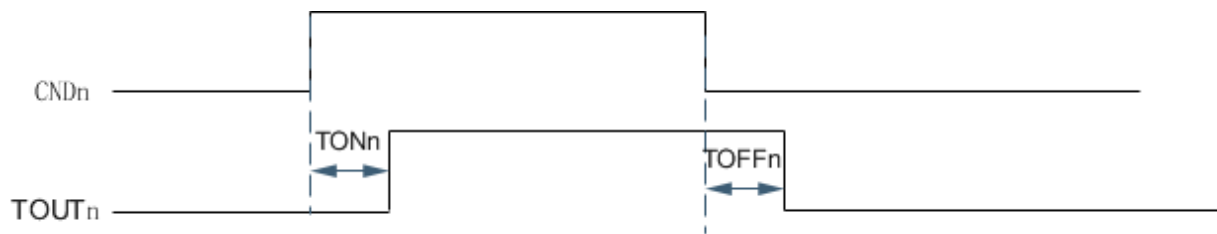
Figure 4.48 The sequence diagram of ITLK_A function block as generating or eliminating delay
